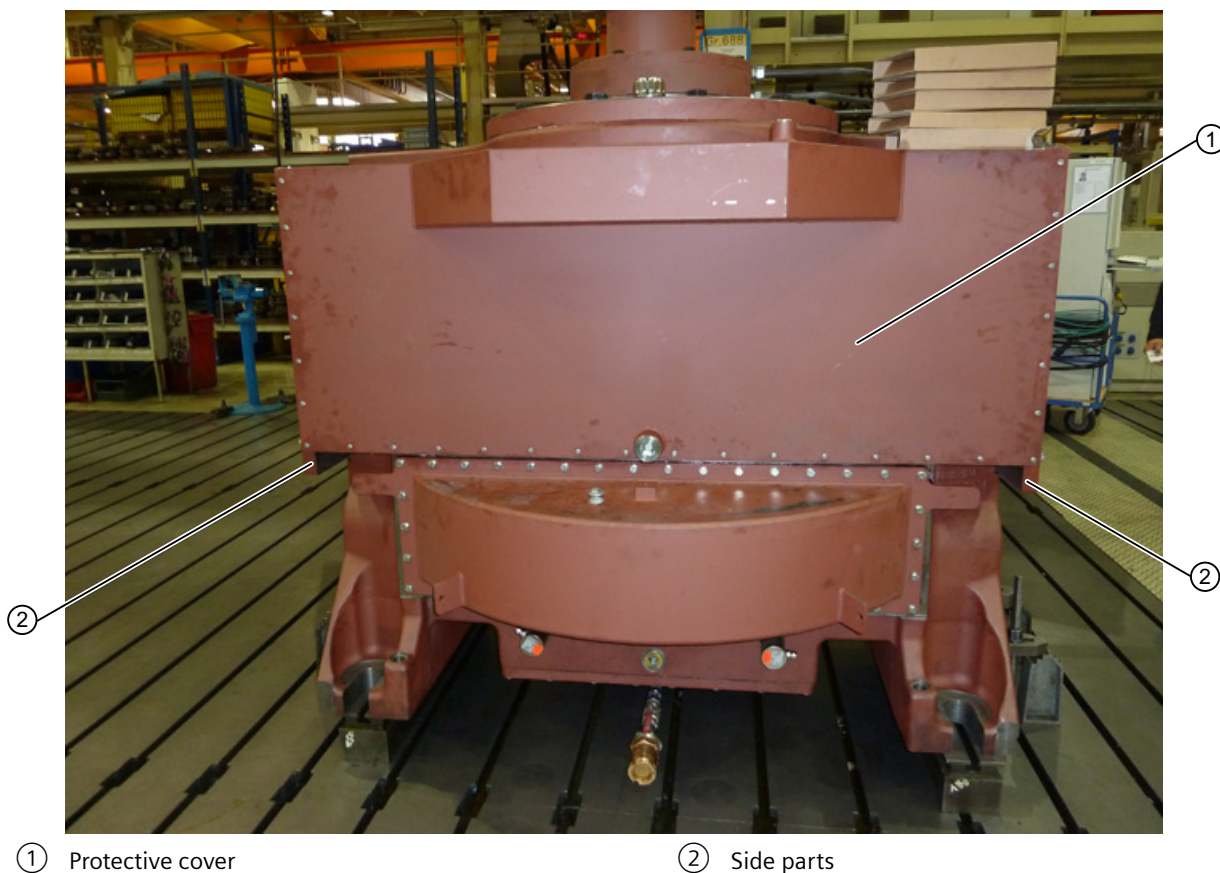
Figure 9-9 Transport cover mounted on the KMRS
