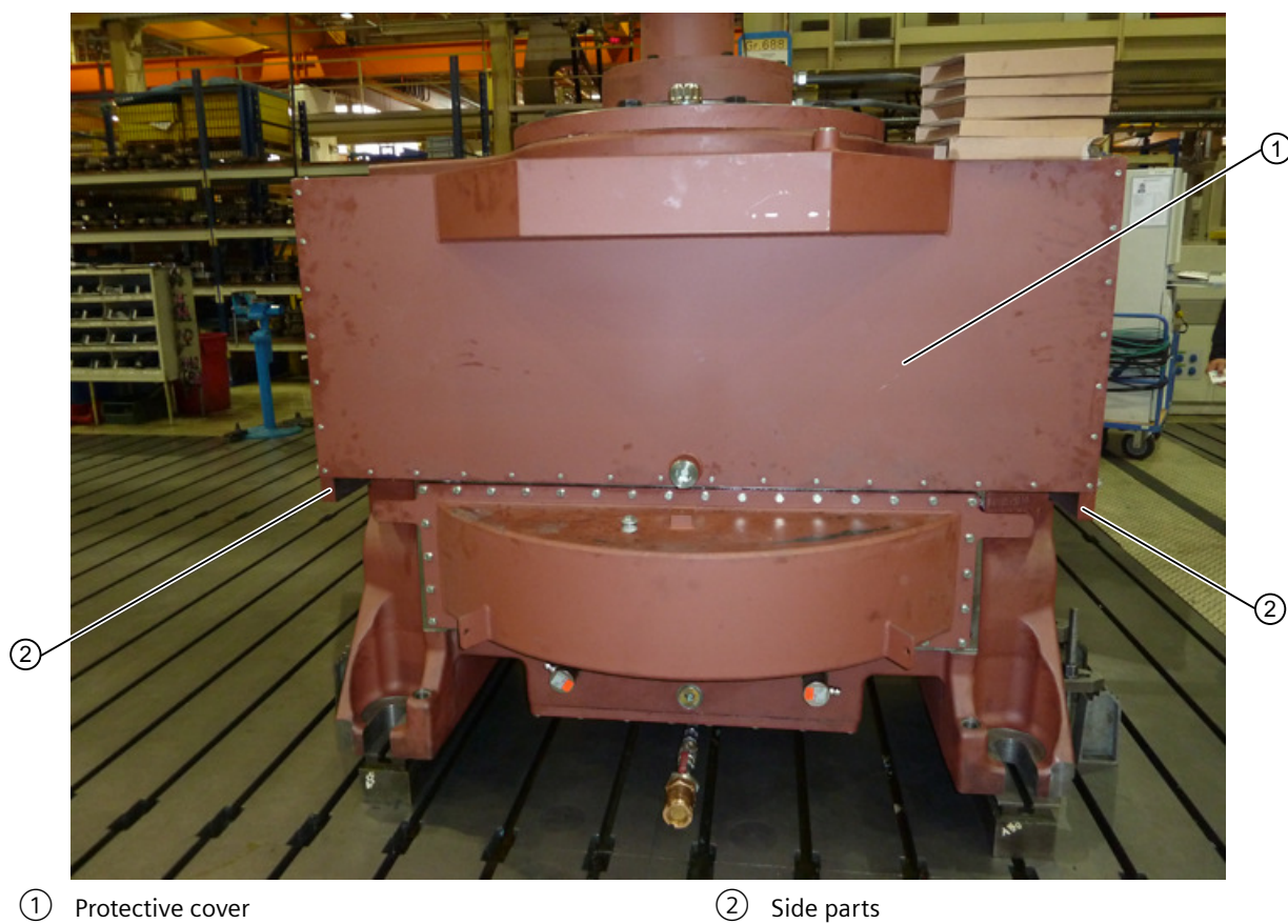
Figure 5-7 Transport cover mounted on the KMRS
