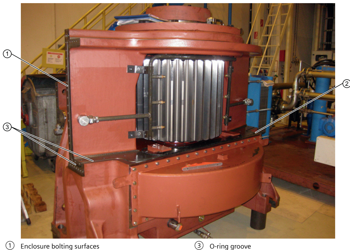
Figure 5-9 Housing bolting surfaces with thread and O-ring grooves
