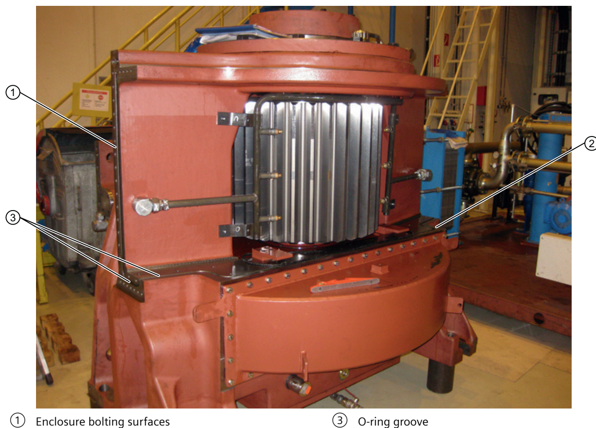
Figure 9-6 Housing bolting surfaces with thread and O-ring grooves
