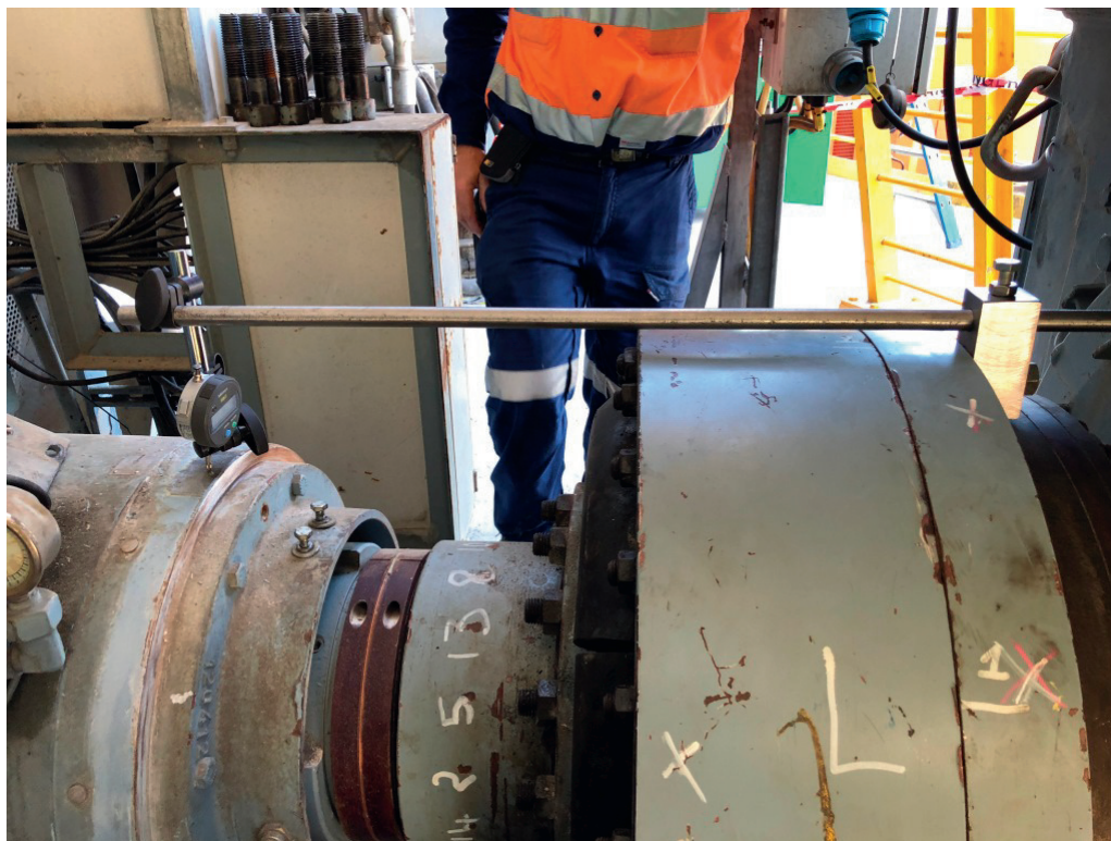
Figure 5-24 Measuring the dimension "a" (radial offset)
