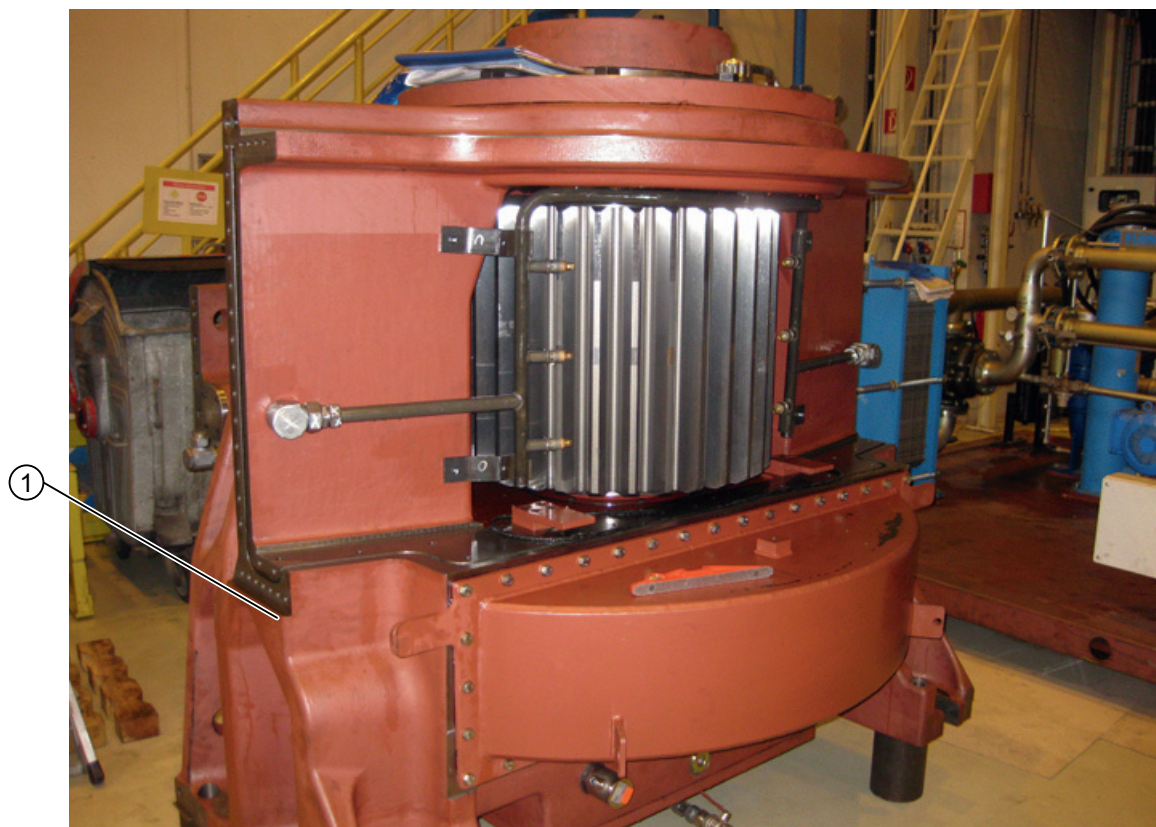
Figure 5-28 The position of the connection threads at the housing of the KMRS to attach the end stops for the limit switches
