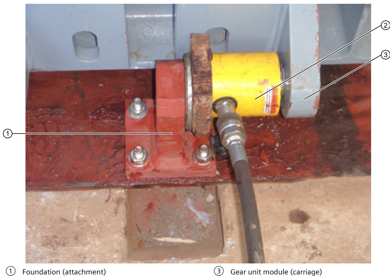
Figure 5-16 Alignment (displacement) of the gear unit module with the hydraulic jack
