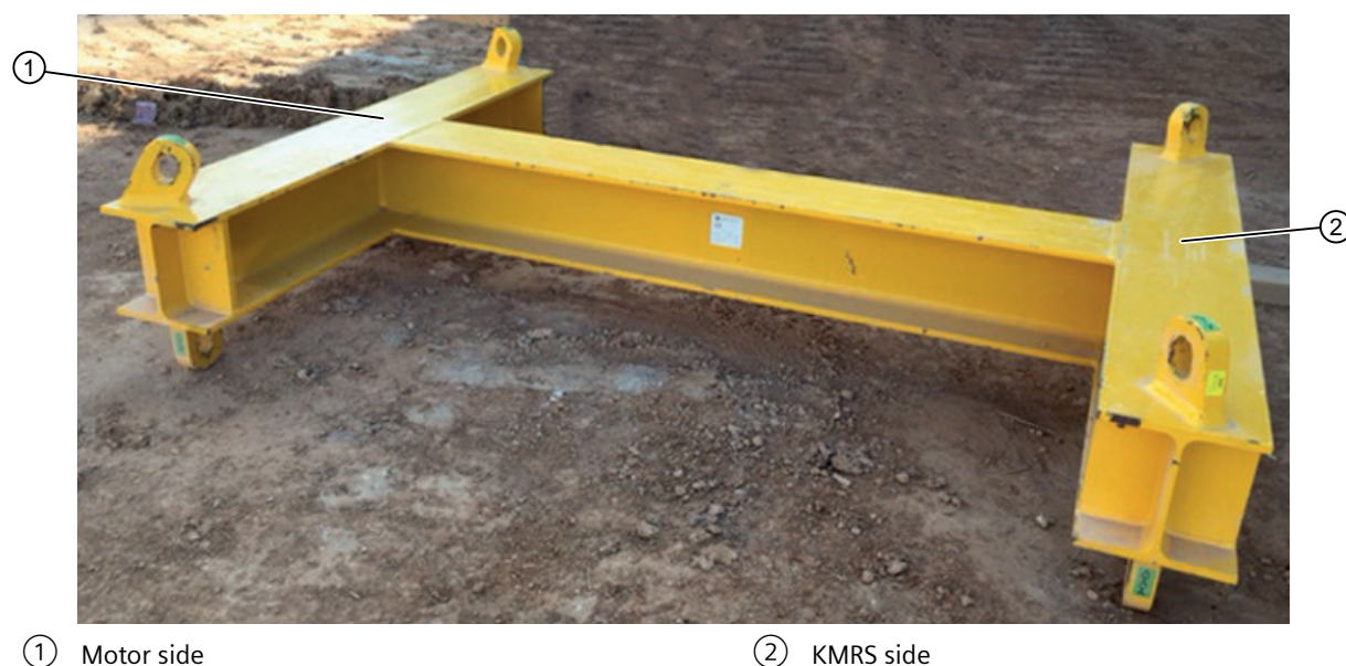
Figure 4-2 Marking on the cross-beam
