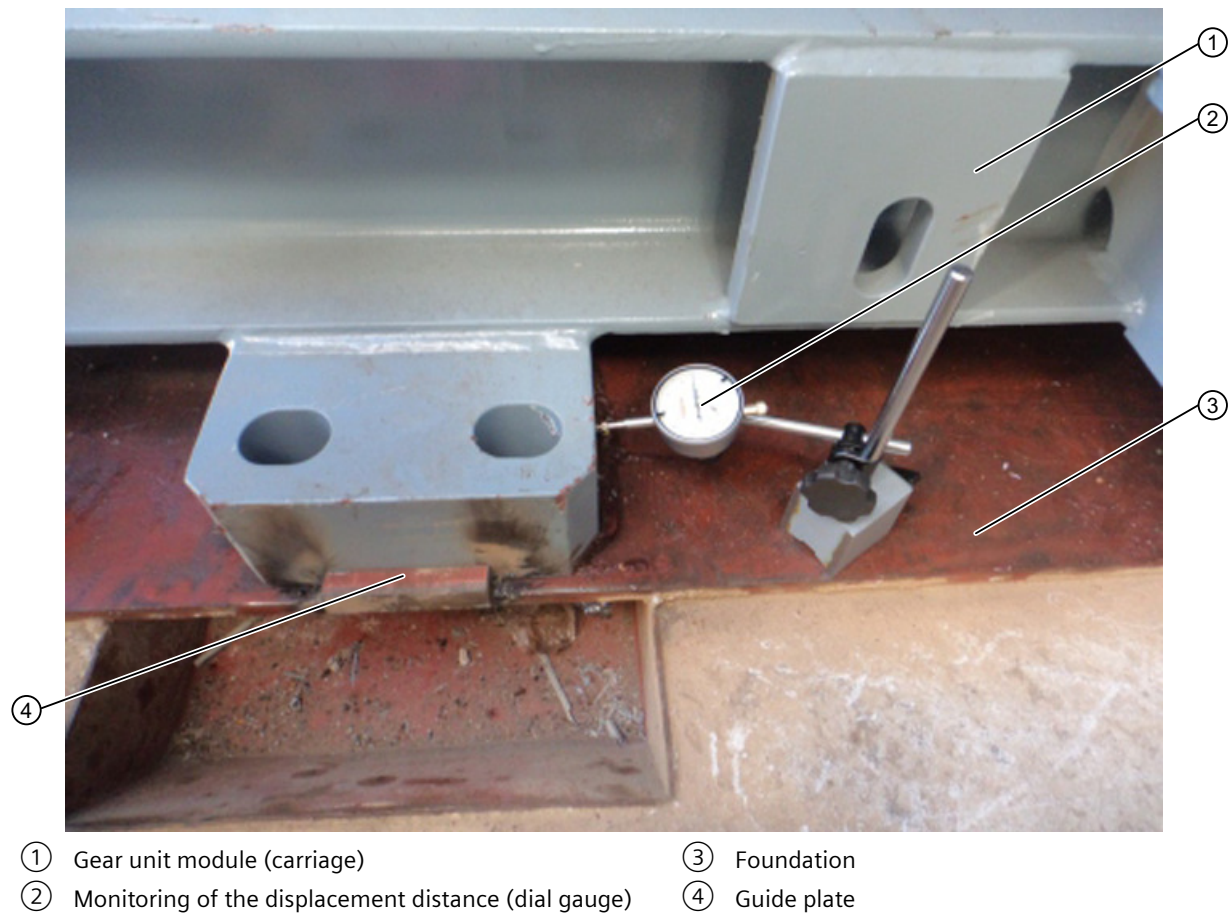
Figure 5-17 Alignment (monitoring) of the gear unit module with the dial gauge
