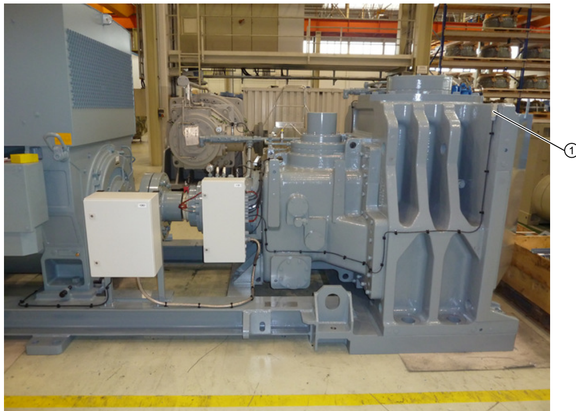
① Plug connection for connecting to the grinding bowl support
