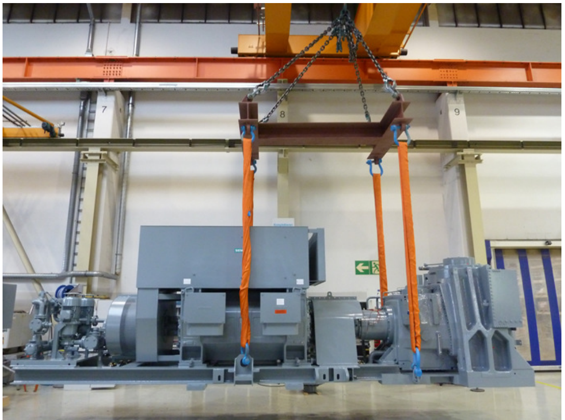
Figure 4-1 Position of the attachment points and transport of the gear unit modules
