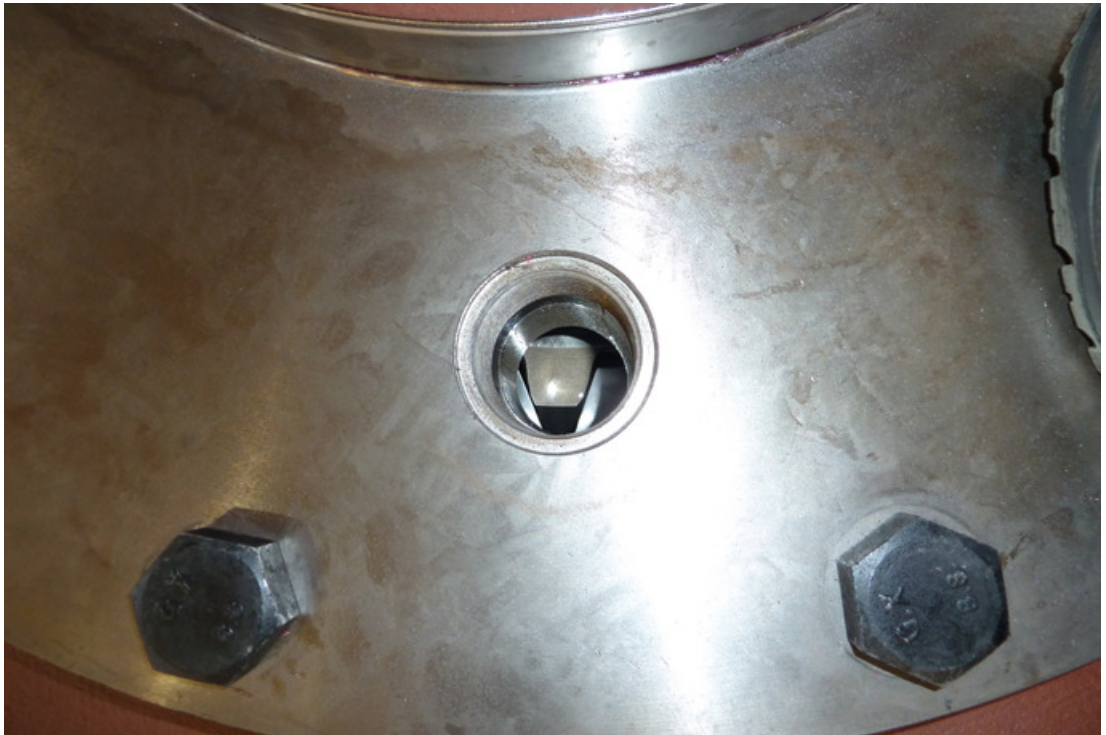
Figure 5-13 Tooth engagement of the pinion at the KMRS with the girth gear
