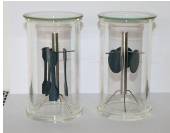
Picture 2: Immersion of samples in test vessel
