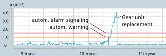
Curve of a damage criterion
