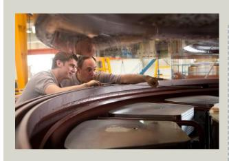
Condition analysis of the respective gear unit on site and identification of the necessary spare parts and required quantity
