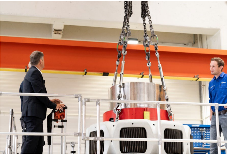
...before he uses a crane to insert the central planet carrier of a real gearbox.
